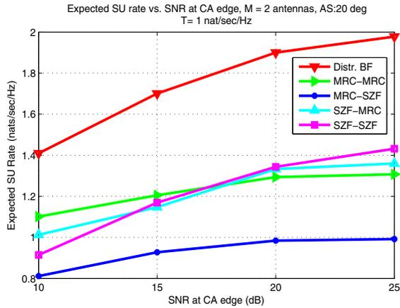
Fig. 2. Expected SU rate vs. average SNR at CA edge.
